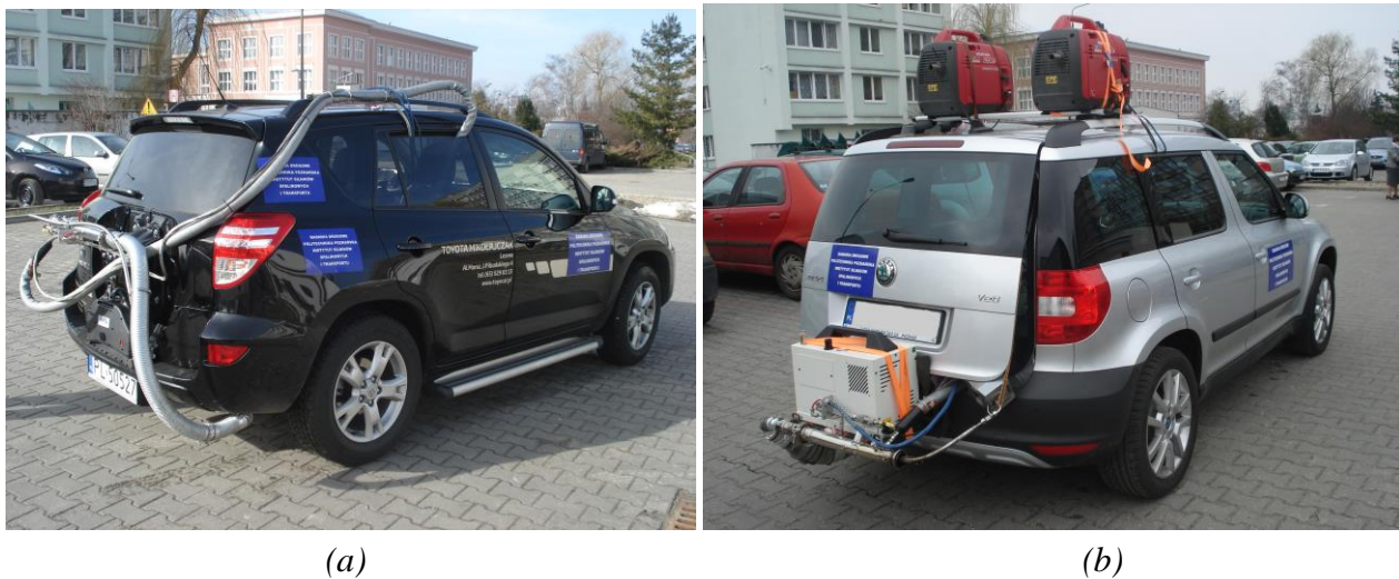
Fig. 1. Exhaust emission analyzers fitted in vehicles A and B during the tests.
